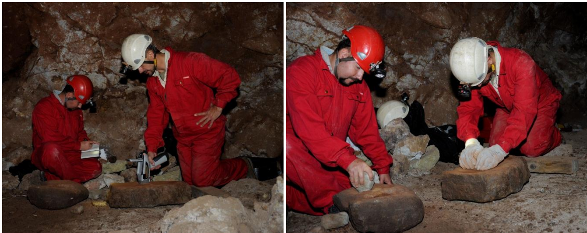
Sampling gold containing ores underground in Sakdrissi by Dr. A. Courcier (Lyon/Bochum) and Prof. Dr. Th. Stöllner (Bochum), right: ore crushing and milling; left: PXRF-measuring.
